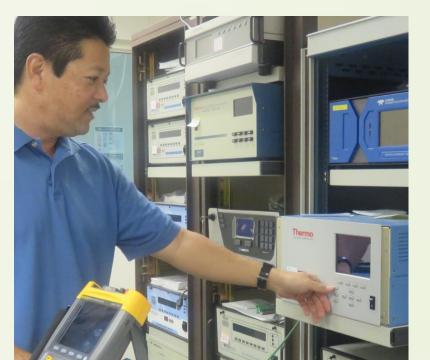
Installed Puna H monitoring station for ambient air pollutants
