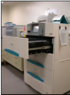
The NH PHL is currently in the process of validating the MGIT 960 for drug susceptibility testing.
