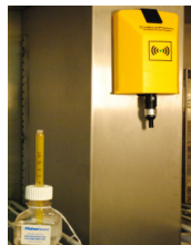
Thermometer and TempSys monitor inside equipment.
