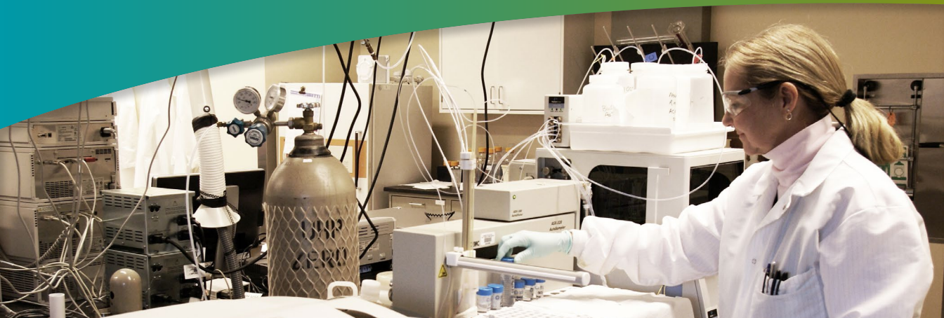
Fran Thompson, senior chemist, analyzing drinking water samples on the Inductively Coupled Plasma-Mass Spectrometer. Photo courtesy of Amy Pierce from the Missouri State Public Health Laboratory.
