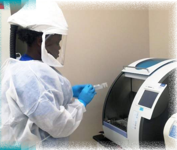
DCLS LRN-Molecular Scientist Asia Bey prepares to setup the MagNA Compact nucleic acid extraction platform for testing in the BT-Bacti Environmental BSL-3 laboratory. The Compact is used routinely for "white" powders, threat letters and MERS-CoV testing at DCLS.
