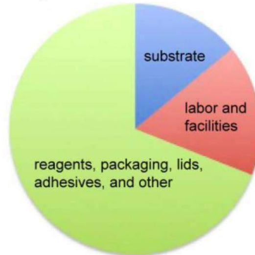
Approximate cost breakdown of Claros plastic microfluidics cartridge
