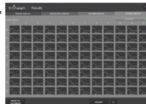
LabChip DS analysis of a 96-well plate of gDNA isolated from different blood volumes using the JANUS chemagic Workstation.
