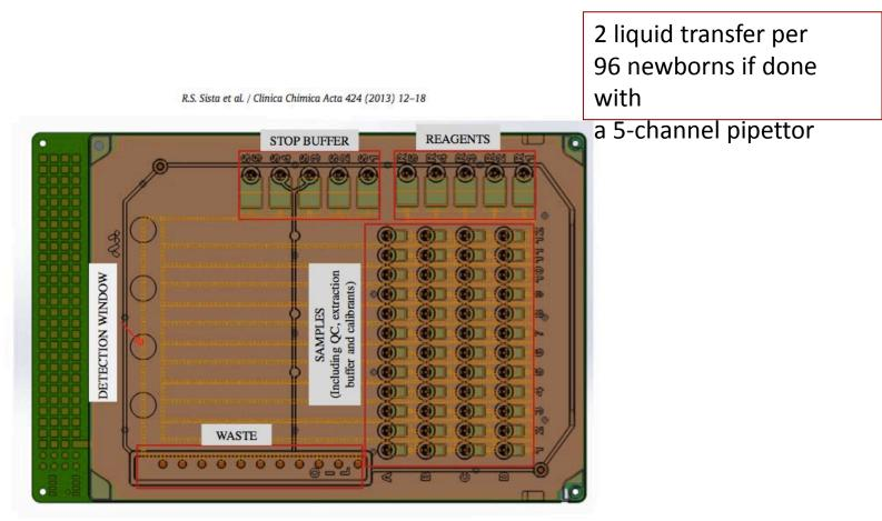
Step 7: Transfer 5 different stop solutions to 5 different reservoirs on chip.
