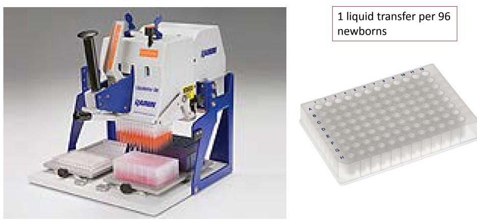
Rainin Liquidator 96-channel pipettor
