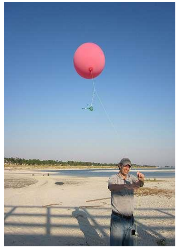
Helium balloon with digital camera attached
